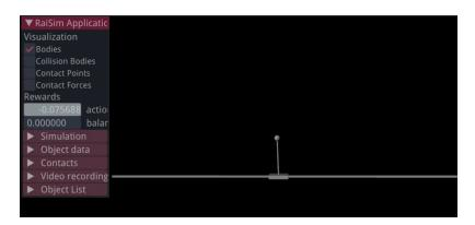
Simple cart pole balancing example using RaiSim.
